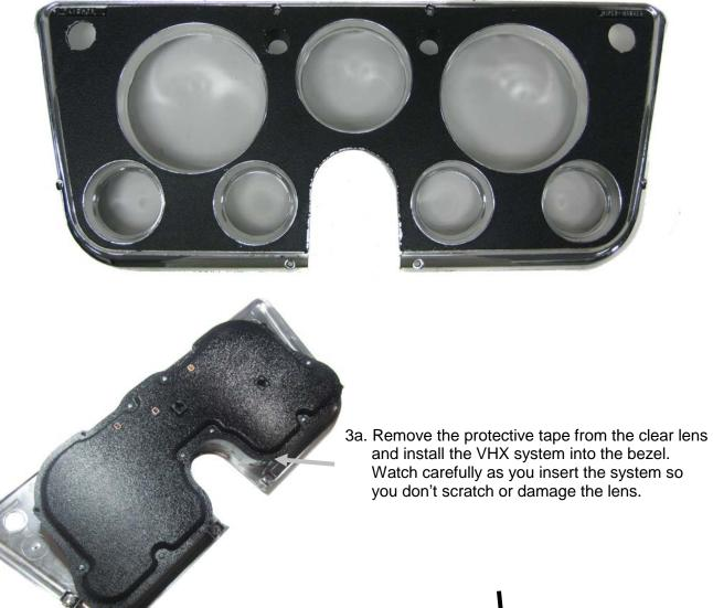
3b. The VHX system should align tightly and the lens should sit flush with the bezel.
