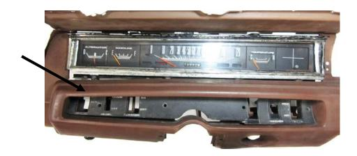
2. Remove the factory gauge cluster from the dash; also remove the gauge cluster bezel from the gauge cluster. Retain all factory hardware for reassembly.
