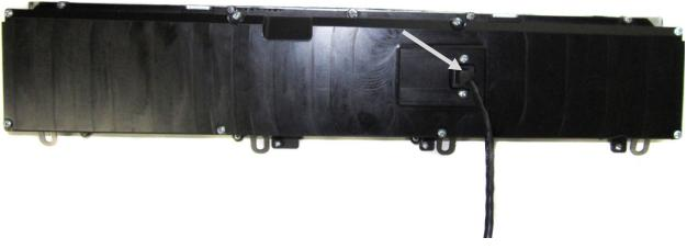
5. Mount the VHX system to the dash using the two (2) factory screws from disassembly for the upper mounts and the provided four (4) oval head screws for the lower mounts.
