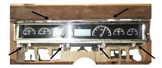
6. Re-install the lower dash pad using the three (3) provided pan head screws. Then mount the switch panel to the dash using the factory hardware from disassembly. Refer to the main manual for wiring instructions to complete the VHX installation.
