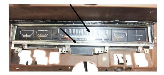
3. Mount the factory gauge bezel to the VHX system by reusing the nine (9) screws that held it to the factory gauge cluster.
