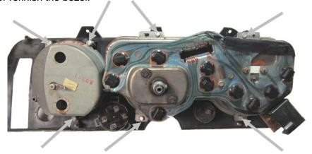
3. Secure the VHX gauges as shown in the picture using the factory hardware. There is adjustment within the mounts so test alignment to the bezel before final torqueing.
