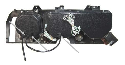
5. This system comes with two options for the turn signals. You can either have arrows located in the faceplate of your new VHX display, and/or arrows in your vehicle's stock turn signal locations. To use the new faceplate arrows, follow the wiring instructions for the turn signals found in the main VHX manual.
