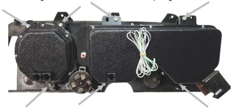
4. Before the assembled cluster is reinstalled, connect one end of the 12" CAT5 cable to either jack on the Tach and the other end to the Speed assembly. Then, connect one end of the 36" CAT5 cable to the remaining open jack on the Tach; use caution when routing the other end of this cable to the control box mounting location.
