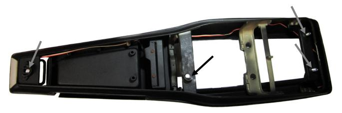
12. Remove the gauge cluster from the console by removing the four (4) screws holding the cluster to the console. Also remove the top screws that hold the bezel to the housing as shown in the picture. The bezel and screws will be reused for the new gauges.
