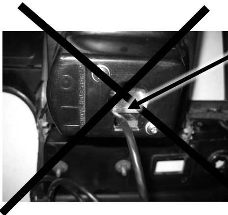
Pre-bend cables to the side before installing so unit will sit flush once inserted into dash
