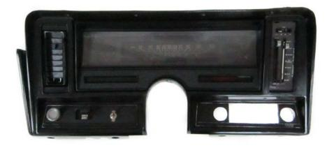
2. Remove the eight (8) screws holding the gauges to the bezel and save the screws for reassembly.
