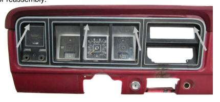
1b. Finally, remove the four (4) mounting screws holding the cluster to the dash. Retain these screws for reassembly.
