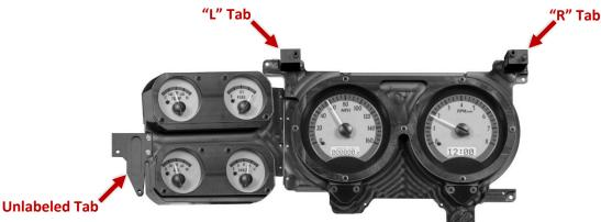
The remaining unlabeled tab goes on the bottom left side of the system, between the satellite gauges. Making sure the countersunk side of the tab is facing away from the rest of the unit, fasten this tab to the VHX system with the two included **6-20 x**  $\frac{34}{7}$  flat head screws. This tab can be tightened until flush.
