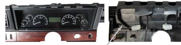
5. Secure the factory lens over the VHX system using the five (5) factory screws. You are now done mounting the VHX system; refer to the main manual for wiring instructions to complete the VHX installation.
