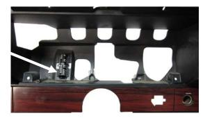
3. Attach the provided 36" CAT5 cable to the back of the VHX system and carefully route the other end to the control box mounting location.
