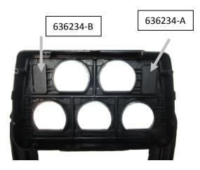
3. Peel the paper off the two block-off lenses needed (636234-A and 636234-B) and place them shiny side down in the two rectangular openings. Use silicone to hold them in place and avoid handling until the silicone has cured.
