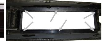
Remove the four (4) screws that mount the stock gauge cluster while retaining the hardware for reassembly, also disconnect the wiring harnesses, shift indicator cable, and speedometer cable to completely remove the gauge cluster. Make sure the harness is pushed back as to not interfere with the VHX mounting.
