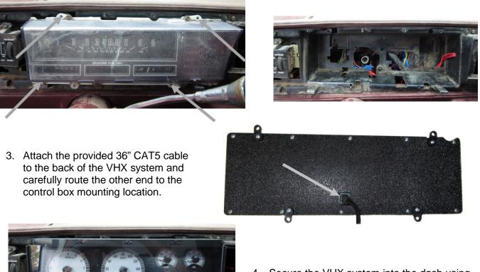
5. You are now done mounting the VHX system; re-install the dash cover and refer to the main manual for wiring instructions to complete the VHX installation.
