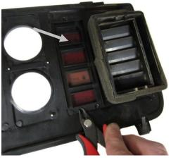
6B. Also the small spacer extrusions on the back side of the bezel will need to be snipped off as shown. Depending on trim level (GT etc) and/or model year, the number of extrusions and locations may vary. Any obstruction from the bezel lying flat against the VHX display needs to be removed.
