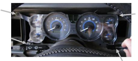
6A. Both the indicator plate and the warning plate will need to be removed from the back of the bezel to allow clearance for the VHX gauges.
