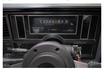
\*The bezel is held in by push-in clips. Note the locations of the clips on the back side of the bezel. Pull near clips when removing the bezel.
