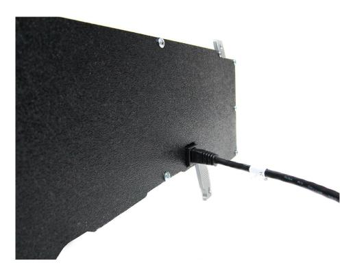
4. Install the VHX system into the dash. Align the four mounting holes and re-use the factory screws to fasten the VHX gauges into the dash.
