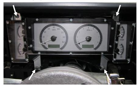
5. Re-install the gauge bezel and refer to the main manual for wiring instructions to complete the VHX installation.
