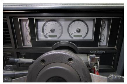
6. Stock charging systems will need an additional wiring connection at the gauge cluster connecter. You will need to add a 300 to 500 ohm resistor between pin 3 (Brown wire) and Pin 15 (Pink/Black wire). The provided alternator load harness can be used to achieve this.
