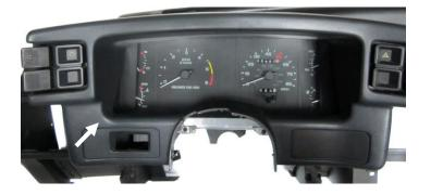
2. Remove the stock gauge cluster by removing the four screws holding the system to the dash structure; be sure to keep these screws as they will be re-used. Now is a good time to clean the bezel and dash pads.
