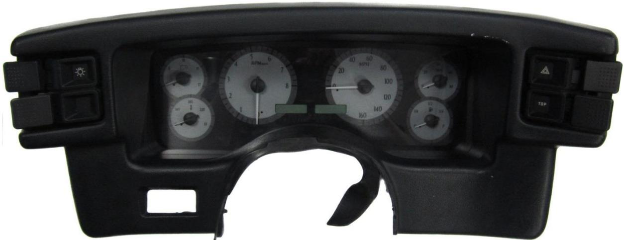
5. Stock Mustang charging systems will need an additional wiring connection at the gauge cluster connector. You will need to add a 300 to 500 ohm resistor between pin 14 (LG/R wire) and Pin 2 (R/LG wire). The provided alternator load harness can be used to achieve this.
