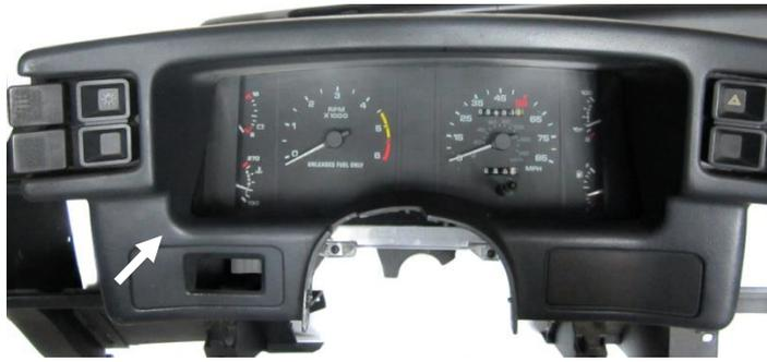
2. Remove the stock gauge cluster by removing the four screws holding the system to the dash structure; be sure to keep these screws as they will be re-used. Now is a good time to clean the bezel and dash pads.
