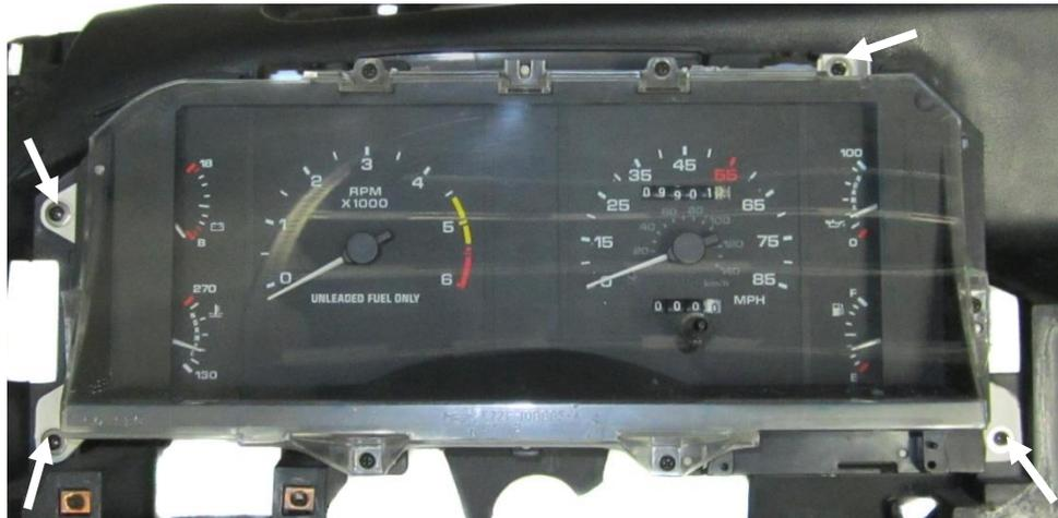
3. Connect the CAT5 cable to the back of the VHX cluster as it is installed into the dash, take care when routing the other end of this cable to the control box mounting location. Mount the VHX cluster to the dash structure using the four factory screws.
