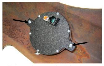
3. Connect the CAT5 cable and switch harness or VLC power harness to the clock and carefully route these back to the VHX control box and refer to the Operating Manual to complete the VHX clock setup.
