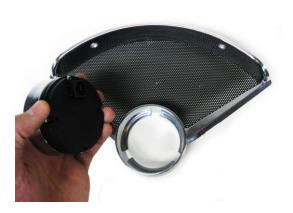
Flip the bezel over. Align the 1/8" thin Clamping Backplate on the back so the connector is at the top, then thread the provided screws into the two locations shown, clamping the system together.
