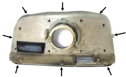
2. Remove the bezel spacer from the factory dash and set aside. The spacer and three screws will be attached to the clock later.
