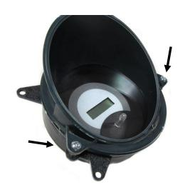
5. With the three factory screws removed in Step Two, attach the assembled clock and bezel spacer to the dash. Connect the CAT5 cable and for VLC's the 12V power harness to the clock and route to the control box.
