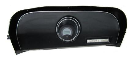
Reinstall the assembly in to the dash and refer to the Operation Manual to complete the clock setup.
