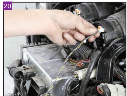
Install the sensor harness 3-pin connector to the 3-pin connector on the speedometer.
