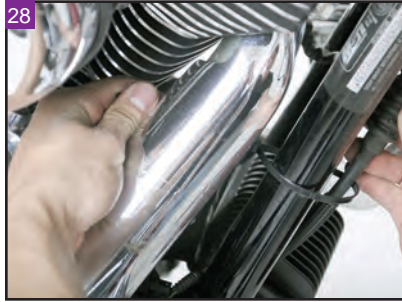
Remove the existing zip tie and secure the harness to the clutch cable with a new, supplied, zip tie and tighten.
