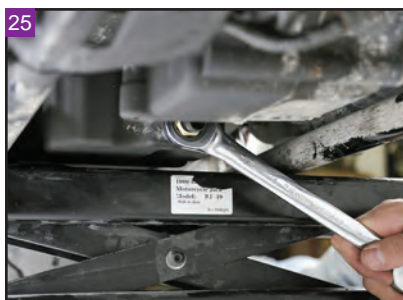
25 Install the oil temp sensor and tighten using a 3/4" wrench.
