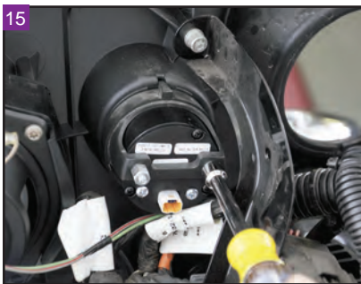
Reinstall the stock mounting hardware and tighten.
