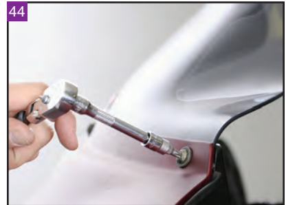
Install the remaining upper mounting screws and tighten.
