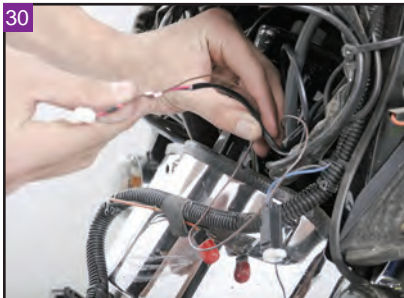
Pull the harness taut through the fairing and up above the stereo caddy.
