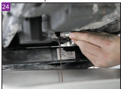
24 Remove the plug. You will have a little loss of oil.
