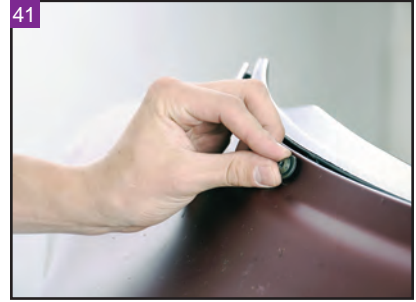
Loosely install the middle mounting screw on the top of the fairing.
