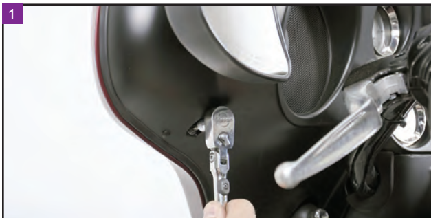
Remove the middle outer fairing mounting screws.
