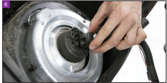
Disconnect the headlight connector.
