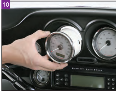
Remove the speedometer and tachometer from the inner fairing.
