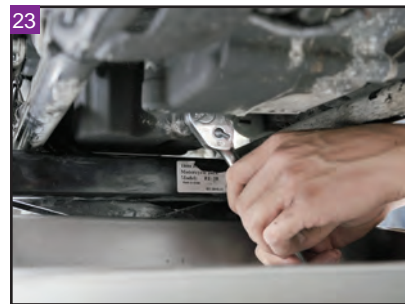
23 Moving to the oil pan, Loosen the 3/8" npt allen plug in the front of the pan. Do not remove the hex plug in the bottom corner for that is your oil drain plug.
