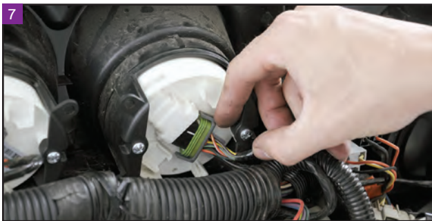
Remove the speedometer and tachometer connector.
