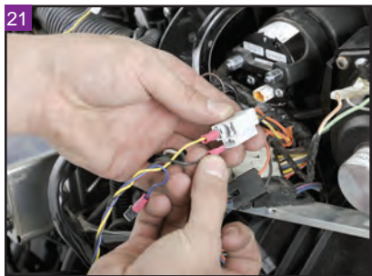
21 Install the yellow and black wire spade connectors to the fuel gauge connector's yellow and black wires.
