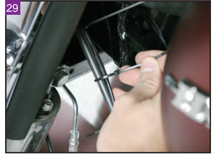
Use the supplied zip ties to secure the harness all the way up the clutch cable, into the fairing.
