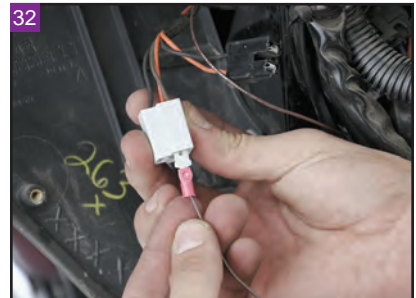
Install the brown wire from the sensor harness into the brown wire on the stock oil psi connector.
