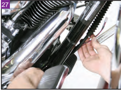
Run the harness along the right frame rail and up the clutch cable.
