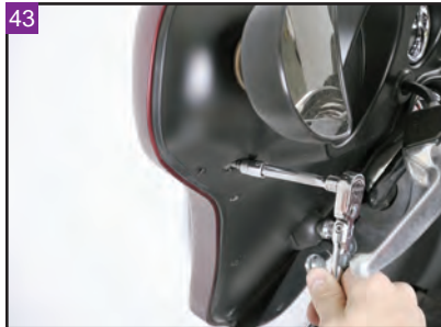
Install the mid level and lower mounting screws and tighten.
