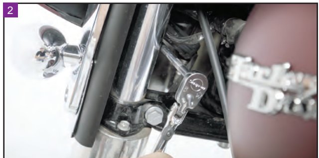
Remove the lower two mounting screws.
