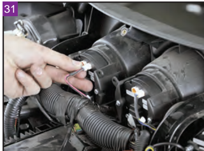
Install the connector in the 3-pin connector on the tachometer.
