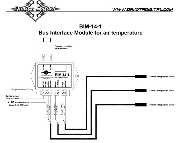
This Bus Interface Module has inputs for up to three digital air temperature sensors, SEN-15-1. Each input can be configured individually. There are two interface ports on the module. Either one can be connected to the gauge system or to another module, allowing several units to be daisy chained together. Do not connect the I/O port to anything other than a Dakota Digital gauge or BIM. Do not mount the module in the engine compartment; it should be mounted in interior of the vehicle.
