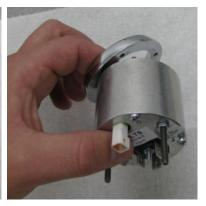
Locate a small black bezel and three of the 4-40 x 1.75" screws. While holding the gauge housing and lens, install one of the screws from the back of the housing through the lens. Hold the screw in place with your finger; carefully align this screw with one of the holes in the bezel to get started, using caution to not scratch the lens.
