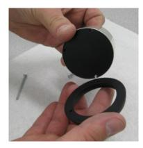
Start one screw a couple turns, do not fully tighten. Align the bezel, pivoting off the one started screw as needed and then start the remaining two screws. Now you can tighten up all three screws, approximately 5.5 in-lbs of torque. DO NOT over tighten!
