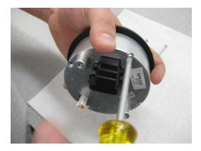
Bezel install is complete, re-install gauge and repeat the steps for the second large gauge.
