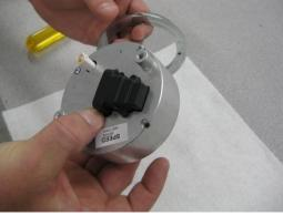
Locate a large black bezel and four of the 4-40 x 1.25" screws. While holding the gauge housing and lens, install one of the screws from the back of the housing and up through the lens, hold the screw in place with your finger. Carefully align this screw with one of the holes in the bezel to get started.
