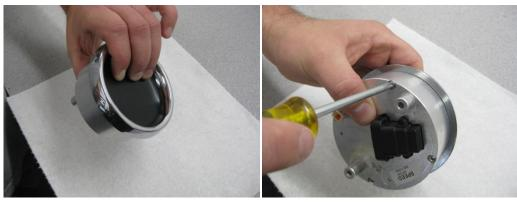
Once the four screws are removed, hold the lens and gauge housing so the lens does not fall out or move. Carefully remove the chrome bezel.
