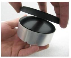
Start one screw a couple turns, do not fully tighten. Use care when aligning the bezel to avoid scratching the lens, pivoting off the started screw as needed, then start the remaining three screws. Tighten up the remaining screws in a criss-cross pattern, approximately 5.5 in-lbs of torque. DO NOT over tighten!
