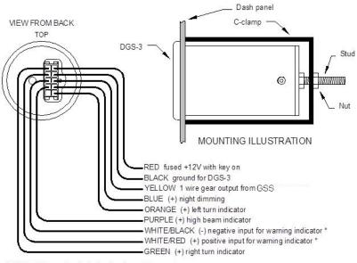
\*NOTE: Both warning indicator inputs must be used.
