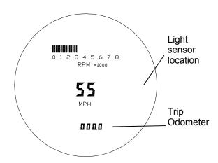
The sealed push button switch supplied with the system will operate the trip odometer. It can be mounted into the hole where the trip reset handle was on your original speedometer. The switch and )-ring go one from the outside of the housing and the retaining bar and self-tapping screw are mounted from the inside of the housing.
