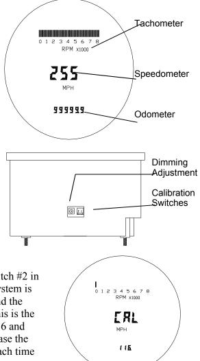
trip/reset button. The number will now increase by one each time the button is pressed. Once the new calibration value is shown, turn power off and then make sure switch #2 is in the on position. The system will now operate normally.
