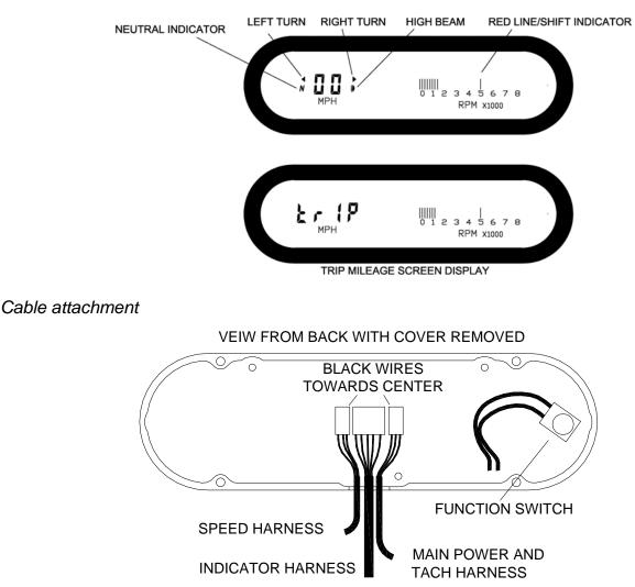
You may want to place a nylon cable tie around the three cables just before they exit the case though the grommet. This will help avoid any stress on the connectors if the cables get pulled during installation or driving.
