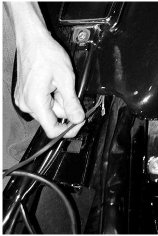
Route wires under tank
