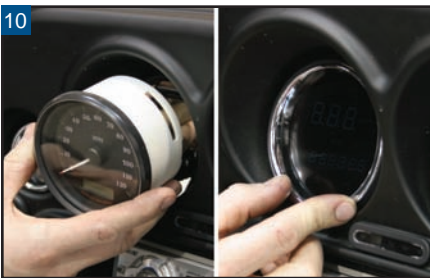
10 Like the previous gauges, the speedometer and tachometer are just as easy to install...
