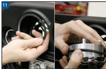
11 ...just make sure the OE weather seal is removed and properly positioned on the new digital gauges.
