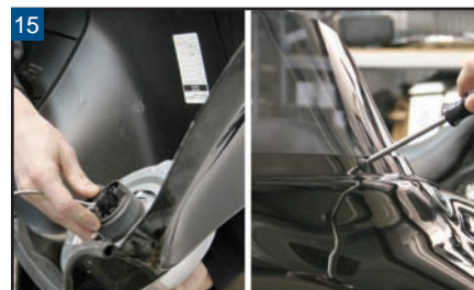
15 Time to plug in the headlight. Reinstall the outer fairing, reconnect the battery and test the new gauges.
