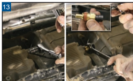
13 Remove the OE oil tank plug from the under-slung oil bag and install the Dakota sensor-sender in its place.
