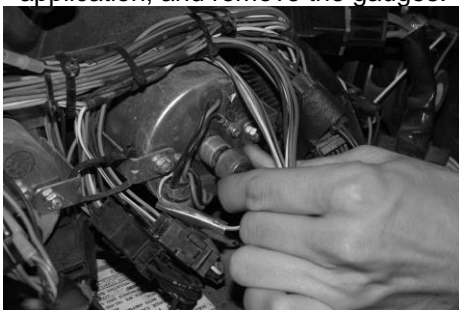
Remove speedo cable/unplug gauges
