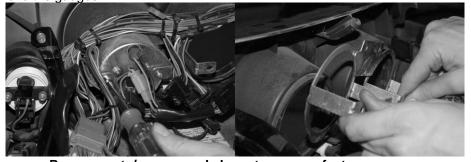
Remove nuts/screws and clamp to remove factory gauges
