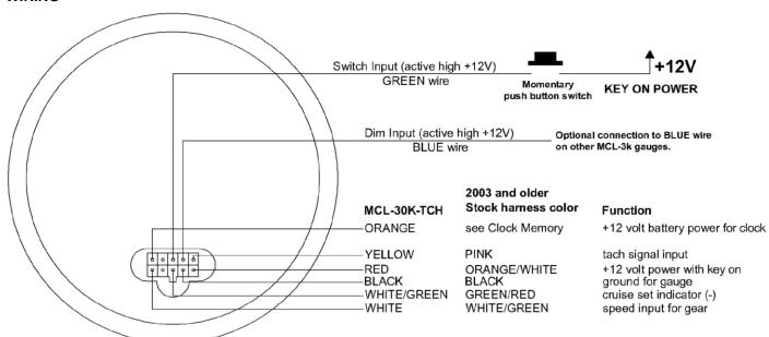
First locate your tachometer connector in the factory wiring harness that were unplugged from the original tach gauge. The wires needed for the Dakota Digital tachometer should all be found here. The factory connector can be cut off or the new wires can be spliced into the harness. Not all wires may be present on all years or models.
