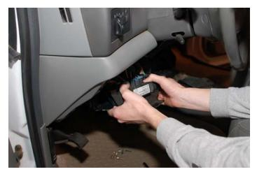
After the 12 volt connection was complete, the negative ground connection was made on a steel support next to the fuse box area.
