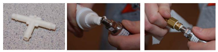
Next, we cut into the factory vacuum line and installed a "T" connector, a short piece of new vacuum line, and the sensor.
