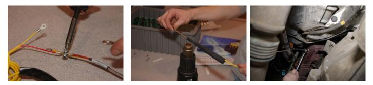
Now it was time for the oil temperature sender installation. We decided not to drill and tap the oil pan for this installation, but instead opted to drill the oil pan drain plug.
