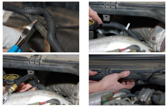
Once the connections were made, the sensor was tied up with the rest of the stock wiring to make for a very clean installation.
