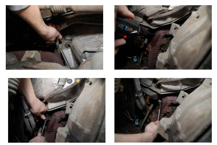
Next, we connected the thermocouple wire extension harness, sealed the connections with heat shrink, threaded the sensor into the adaptor on the manifold, and routed the wire up into the engine compartment.
