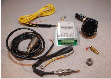
The gauge installation was fairly straightforward and as always with any electrical installation we started by disconnecting the vehicle's battery negative connection as a safety precaution. Next, we started looking for a suitable location to mount the sensors. The turbo boost sensor needs to be connected to a main vacuum line, we found a suitable location near the turbo on top of the engine near the firewall.
