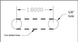
Once the hole is cut insert the button panel from the front. From the back, slide the two L-clamps over the studs and secure with the supplied lock washers and nuts.
