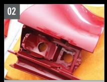
We began by removing the rear taillight assemblies and the bulb sockets. This was an excellent time to carefully inspect the housing for any needed repairs or replacement.
