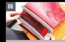
Taillight lenses and housings are not included in the kit. Dakota Digital suggests you inspect them carefully and replace any parts that can not be cleaned or repaired.
