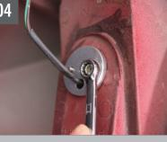
A backing plate was then placed on the backside of the taillight assembly and secured using the provided self locking hex nuts. Tighten evenly working side-to-side.
