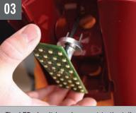
The LED circuit boards mount to the taillight assemblies using the original bulb socket hole. The machined aluminum post extends the LEDs close to the lens.
