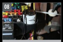
The change in load on the flasher may cause the taillights to not signal properly. Using this "no load" flasher, available from Dakota Digital, will remedy the situation.
