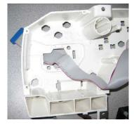
Use the four original screws to secure the Dakota Digital system to the housing.
