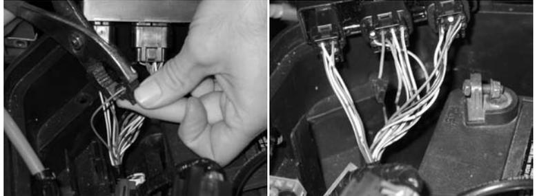
8. Route the wires from the UTV gauge through the hole in the gauge opening and place gauge into opening. Secure the gauge with the three provided washers and thumb nuts.
