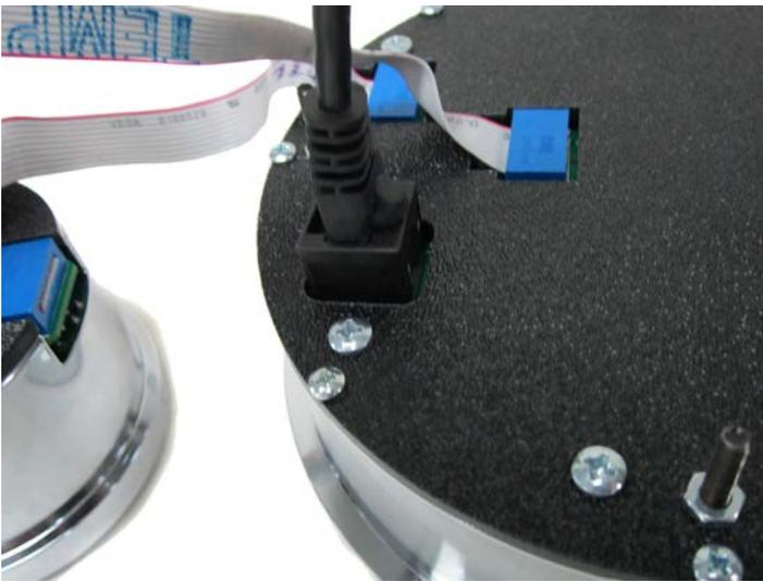
5. Connect the CAT5 cable to the backside of the large gauge and take care when routing this cable to the control box mounting location.
