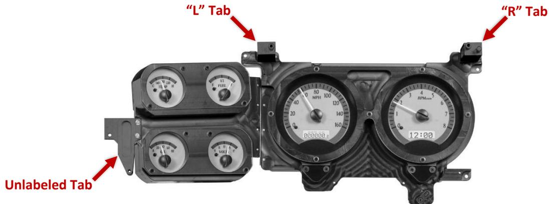
The remaining unlabeled tab goes on the bottom left side of the system, between the satellite gauges. Making sure the countersunk side of the tab is facing away from the rest of the unit, fasten this tab to the VHX system with the two included **6-20 x ¾” flat head screws**. This tab can be tightened until flush.
