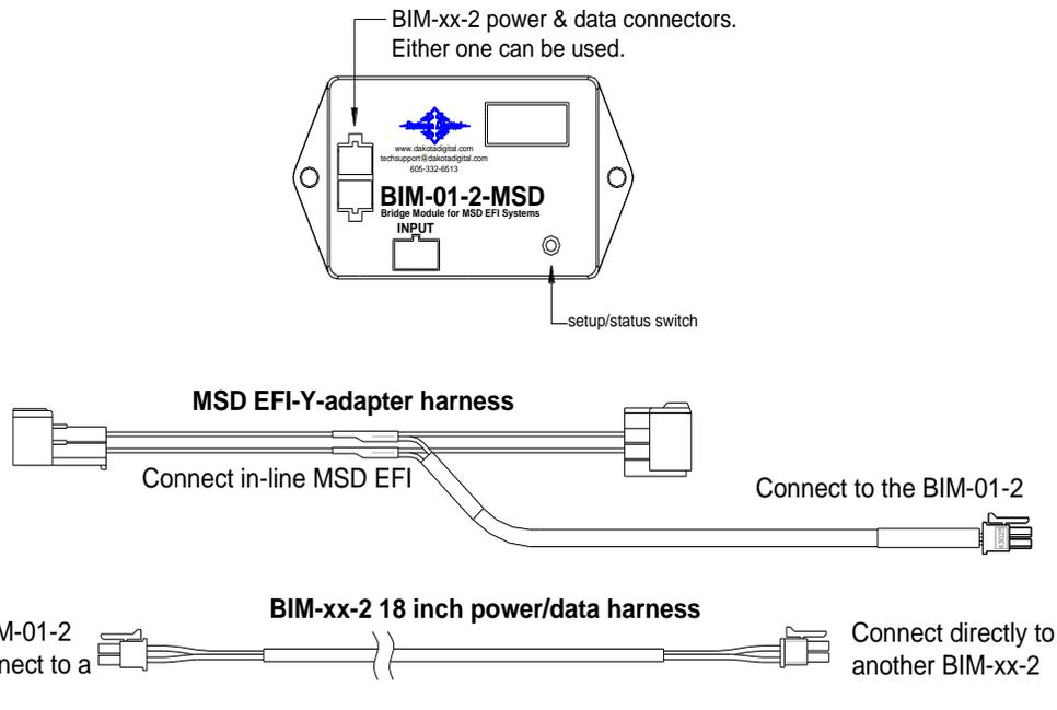
This Bus Interface Module is designed to read engine information from MSD Atomic EFI TBI kits. Atomic EFI LS is not compatible. This module is connected to the MSD EFI through the included Y-adapter harness. This can be plugged in line with the Atomic handheld display or the throttle body.
