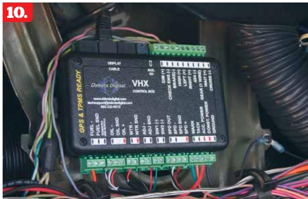
**10.** Using a combination of the Dakota Digital instructions and the Ford wiring diagram, the factory wires for the high beam, turn signals, dash lights, ground, fuel gauge sender, 12V constant, and key on power, along with the new wires from the Dakota Digital harnesses for the oil, temp, and speed sensors, were all hooked up to the control box. The bulk of wiring under the control box is the factory Ford wiring without the wrapping.
