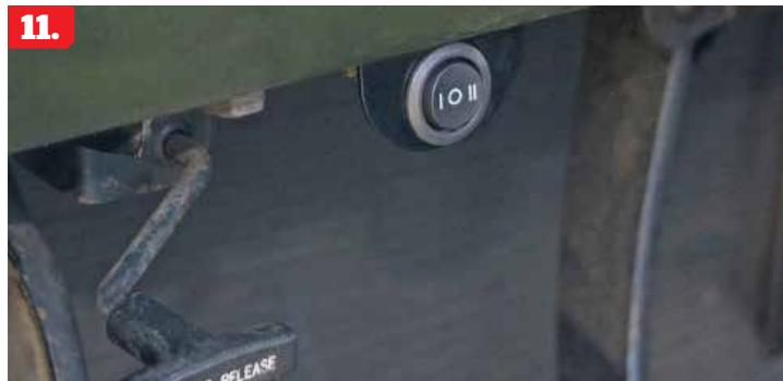
**11.** The kit comes with this switch and bracket, which is used for programming the gauges and for toggling between different functions. We mounted it under the dash on the left side.
