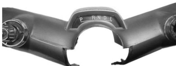
8. With the lower dash bezel already out, remove the two mounting screws to remove the indicator plate and lens.
