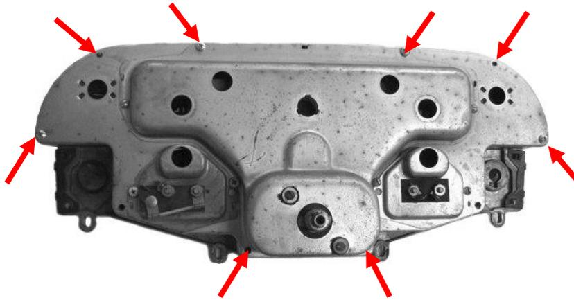
3. Remove all lens and separator plates from the bezel. The odometer lens and gear indicator lens will need to be drilled out. You should be left with a bare bezel.
