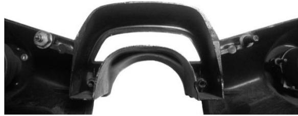
9. Peel off the protective paper and lay the block off lens flat in the gear indicator opening. Use silicone to adhere the lens to the lower dash bezel.
