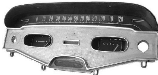
2. Remove the stock gauge housing from the bezel by removing the (8) eight screws on the rear of the metal housing. The only item to be reused is the original front bezel; the other pieces can be discarded. Now is a good time to clean or refinish the bezel.
