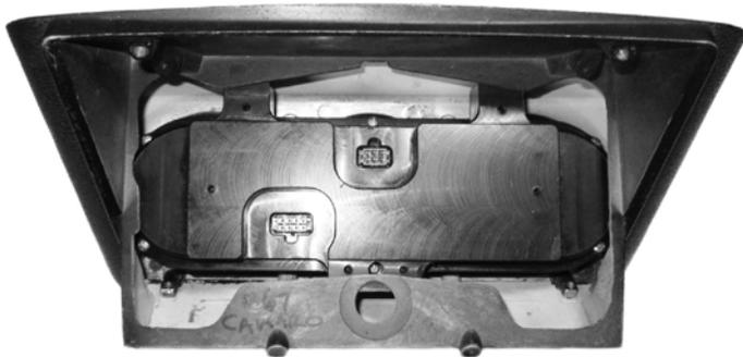
12. Align the bottom portion of the console housing over the back of the VHX console system and mount the two halves of the housing back together with the factory screws.
