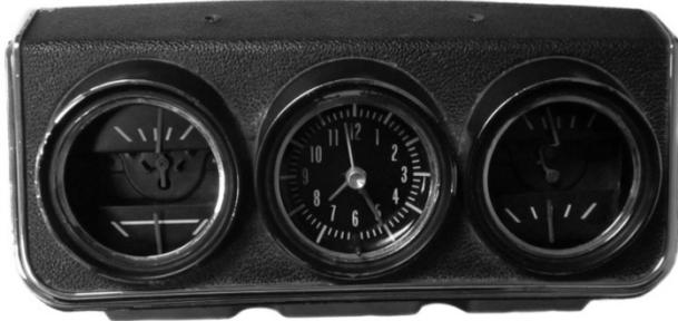
9. Remove the console gauge assembly from the console.
