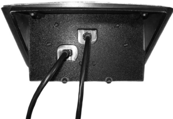
14. Connect the clock harness and the other main harness to the back of the assembled cluster and carefully route the other ends to the Control Box mounting location.
