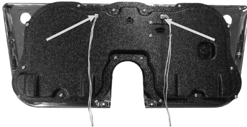
5. Connect the provided main harness, clock harness, and the buzzer (optional for audio feedback) to the back of the HDX system.
