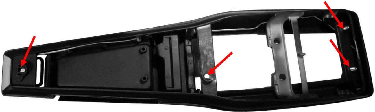
10. Remove the gauge cluster from the console by removing the four (4) screws holding the cluster to the console. Also remove the top screws that hold the bezel to the housing as shown in the picture. The bezel and screws will be reused for the new gauges.
