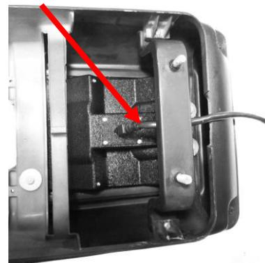
13. Connect the provided Y harness to the Control Box so both main harnesses can be connected.
