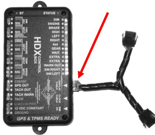
14. Carefully route both main harnesses to the control box mounting location and connect to the Y harness; refer to the main manual for wiring instructions to complete the HDX installation.
