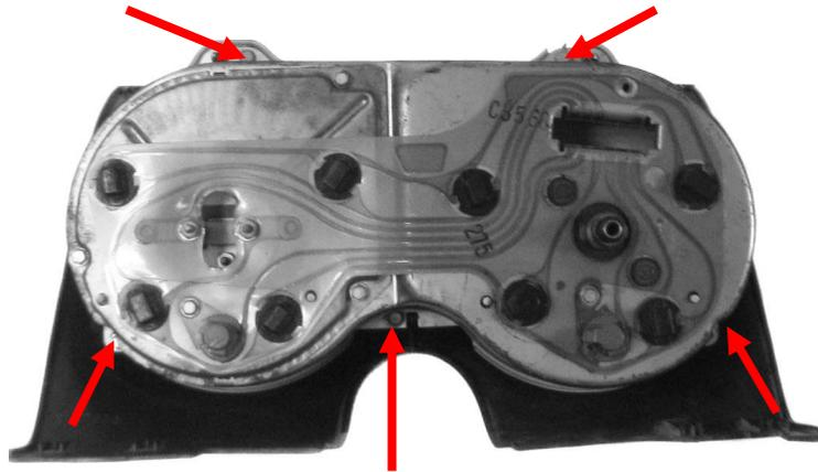
3. Remove the stock gauges and lens from the bezel
