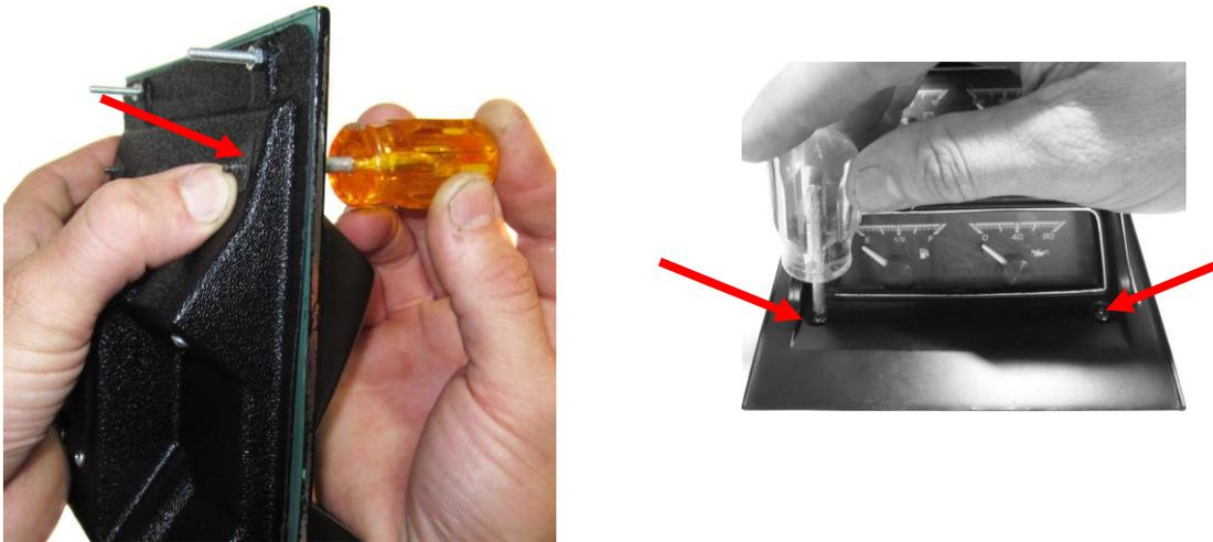
12. With the bezel mounted to the HDX system, align the cluster back into the console and use the provided four (4) fender washers and thumb nuts provided to secure the cluster to the console. Also connect the final main harness to the back of the HDX system. The console is now ready to reinstall back into the vehicle.
