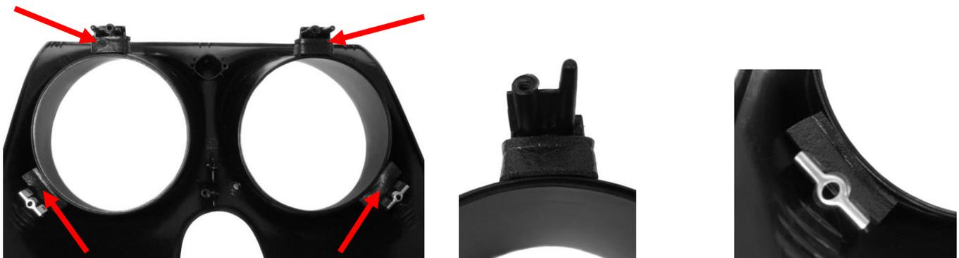
On the top two locations, fold the foam over the edges and make sure it's not sticking into the visible window. In the bottom two corners, the area for the tape is slightly narrower than the foam so you will need to ensure the foam is curved with the opening in the housing.
