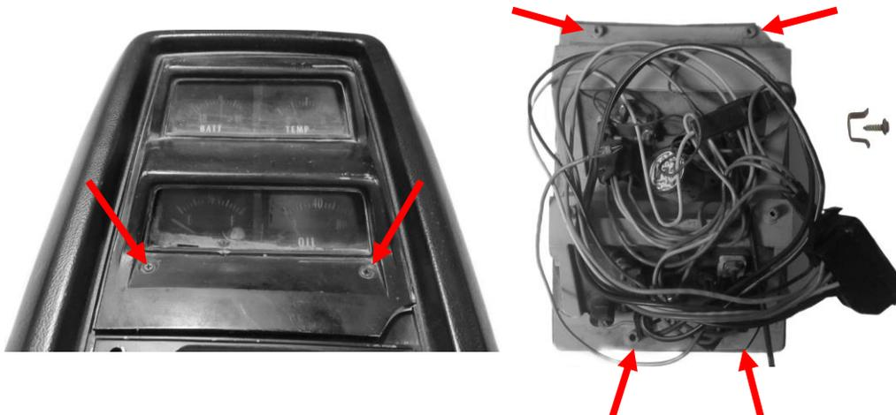
11a. Place the bezel over the HDX system and be sure to align the tabs from the bezel into the slots cut into the HDX housing as shown.
