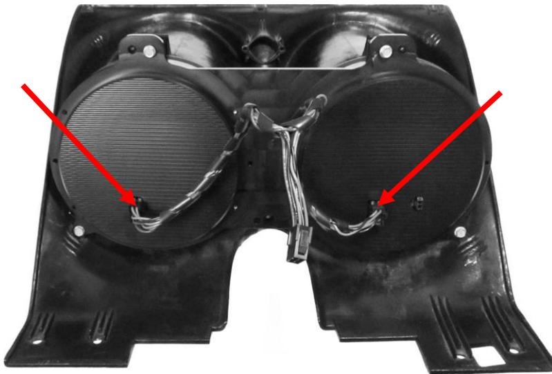
7. Connect the provided harness and the buzzer (optional for audio feedback) to the back of the HDX system.
