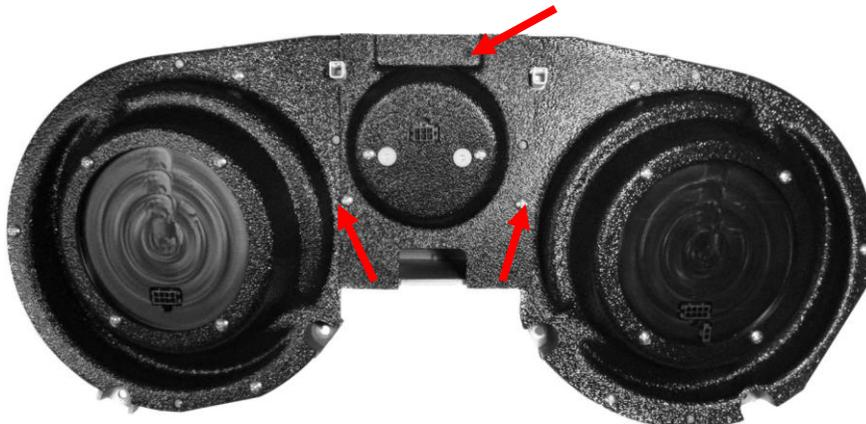
5. This system comes with the option to use two sets of turn signals in your dash: arrows located in the faceplate of your new HDX display, and arrows in your vehicle's stock turn signal locations. To use the new faceplate arrows, follow the wiring instructions for the turn signals found in the main HDX manual.
