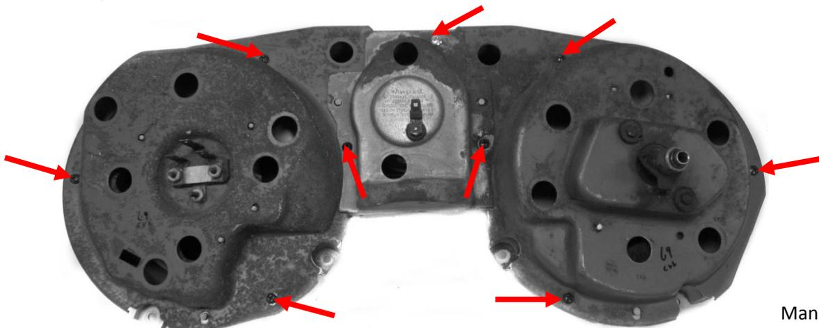
2. Remove the stock lens using a pair of side cutters or a utility knife; the original lenses will not be reused. Using a small flathead screwdriver, remove the clock adjustment screw to allow lens to be lifted off of the housing (Fig. 2b.)
