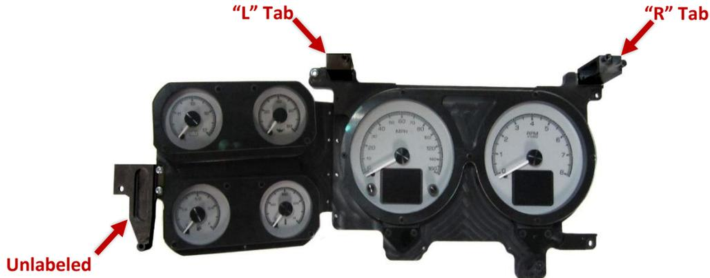
The remaining unlabeled tab goes on the bottom left side of the system, between the satellite gauges. Making sure the countersunk side of the tab is facing away from the rest of the unit, fasten this tab to the HDX system with the two included **6-20 x 3/4” flat head screws**. This tab can be tightened until flush.
