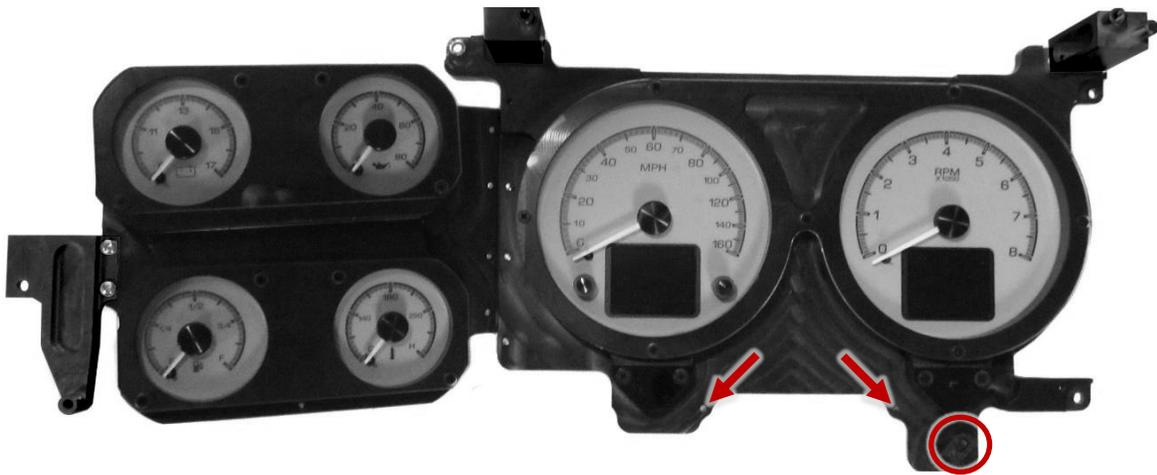
7. Install the stock bezel over the HDX gauge cluster using the stock screws removed in Step One. Tighten the locations shown below first to ensure proper fitment and alignment; if the holes are not aligned correctly, Step Three may need to be repeated.
