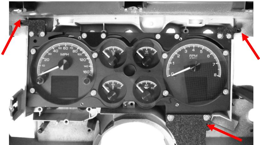
8. Separate the stock lens from the blackout plate; the original lens is not needed. Place the blackout plate over the Dakota Digital gauges while aligning the mounting holes. Attach the HDX system using the five factory screws. Place the included 1/8" white plastic spacer beneath the blackout plate at the lower-most mounting hole before installing the screw (white arrow).
