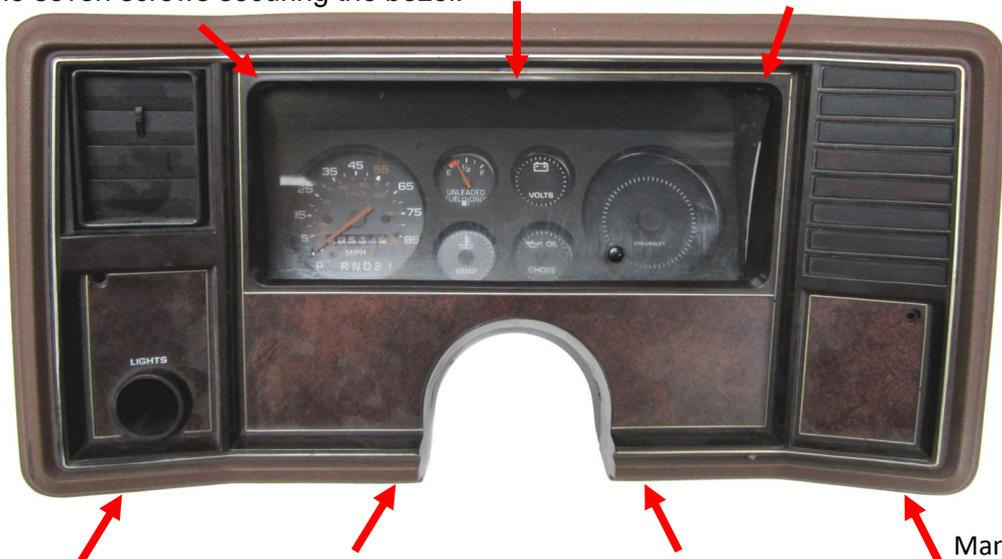
2. Remove the six screws securing the blackout plate and lens to expose the factory gauges. These screws will be reused.
