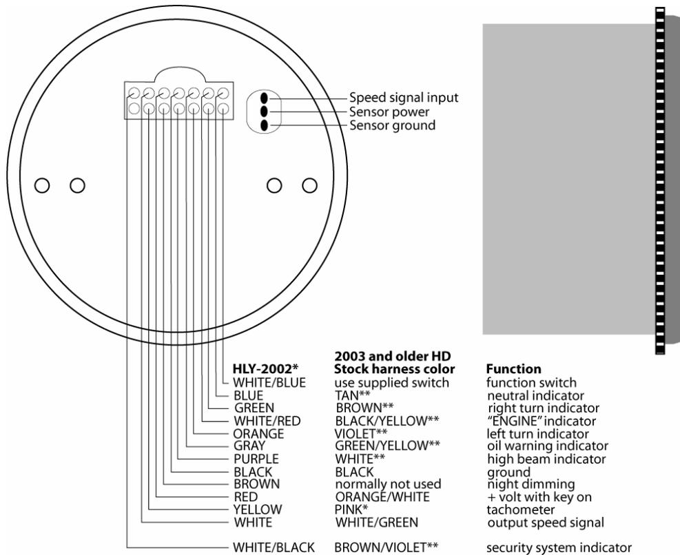
**\*To avoid damage to motorcycle**, please see Speedometer, Tachometer, and Status and Warning Indicators sections for details on locating VSS, Tachometer, and indicator wires for **most motorcycle applications**
