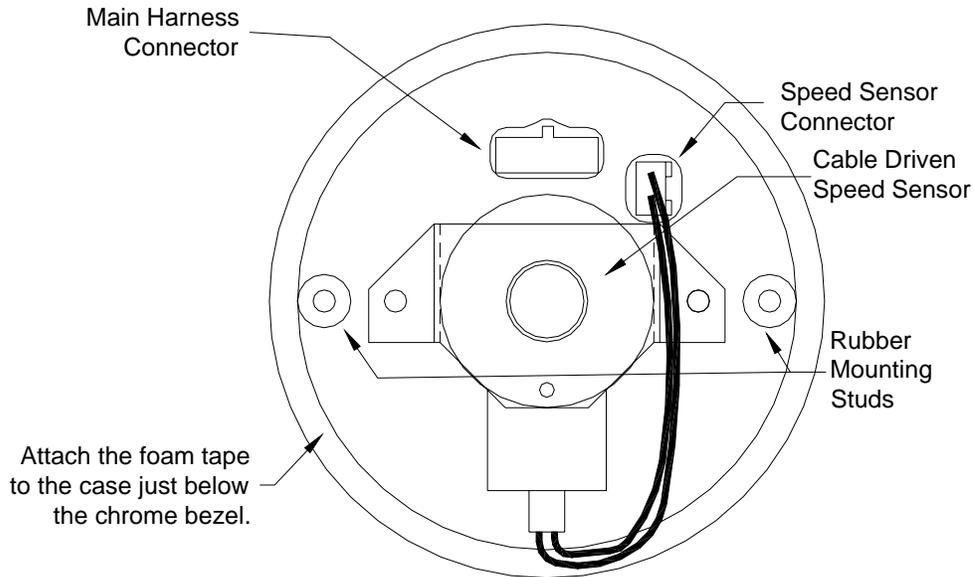
Mounting hardware and speed sensor connection for the clip-in system with an electric, transmission speed sensor.
