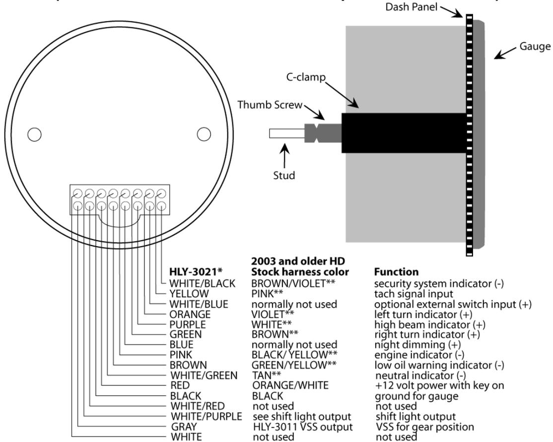
**\*To avoid damage to motorcycle**, please see Tachometer and Status and Warning Indicators sections for details on locating Tachometer and indicator wires for **most motorcycle applications**
