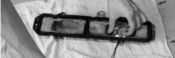
7. Feed the wires through the larger hole in the mounting plate and guide it to the bottom of the housing. The flat side of the mounting plate should be on the outside of the housing and the side with the slight raised center should go into the tail light housing. This will properly align the mount in the original housing.
