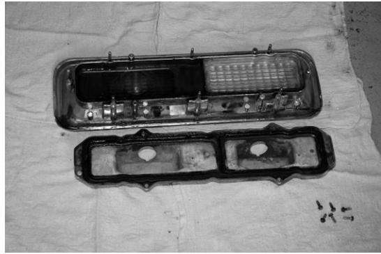
4. Now is a good time to clean the lens and housing. If lenses are in bad shape a new set is recommended.
