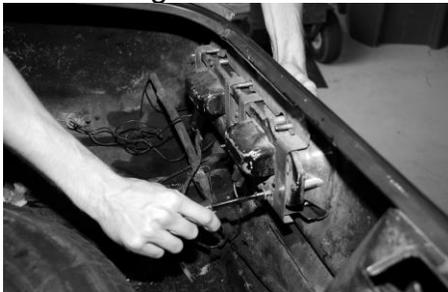
3. Next remove the lens to gain access to the housing. There are six screws that hold the housing halves together, remove the screws and separate the halves carefully.
