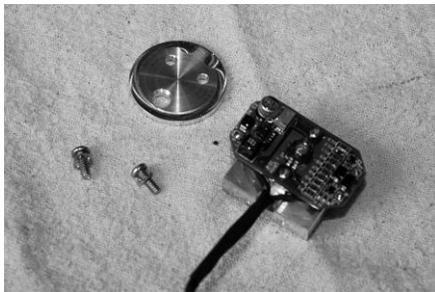
6. Pass the wires through the housing where the original bulb and socket were.
