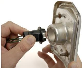
2. Remove the tail light housing hardware so the housing can be taken out of the car. Remove the housings from the vehicle carefully so the body gaskets are not damaged.
