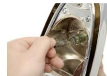
4. Now is a good time to clean the lens and housing. If lenses are in bad shape a new set is recommended.
