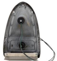
9. Make sure the original lens gasket is in place and replace the taillight lens. Tighten the screws down carefully. Replace the chrome trim pieces.
