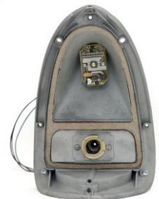
7. Guide the wires through the plastic back plate and slide the back plate onto the stud sticking out the back side of the housing. **Ensure wires are not pinched to avoid shorting!**
