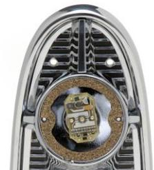
7. Insert the wires through the aluminum spacer, with one wire going through each one of the outer holes. **Ensure wires are not pinched to avoid shorting!** Slide the aluminum spacer over the stud through the hole in the center of the spacer, shoulder side toward the back of the tail light bezel.
