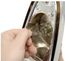
4. Now is a good time to clean the lens and housing. If lenses are in bad shape a new set is recommended.
