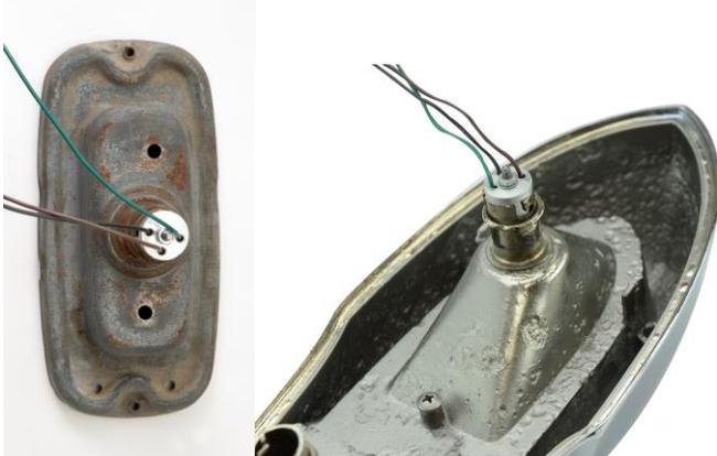
9. Place the original lens gasket into place and replace the tail light lens. Tighten the screws down carefully.
