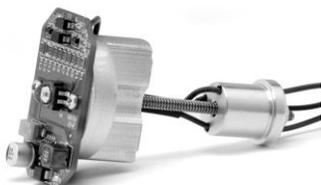
6. Insert the new LED assembly through the hole where the original bulb and connector were. Use caution when feeding the wires through to avoid damaging the wire insulation.
